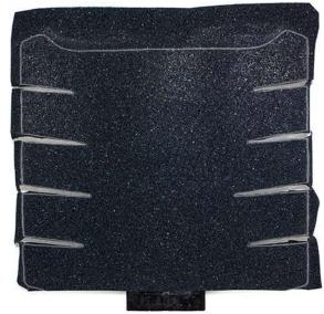
Tear the grip tape edges to ensure you can file the inside the fins.
