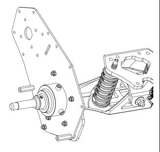
Align drive perpendicular to square hanger base. Tighten up screws bit by bit in correct order! Start with M5 grub
