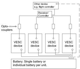
Multiple VESC controllers connected to one receiver or micro controller via CAN. Receiver or controller can be powered from any source. Only connect CAN H and CAN L.
