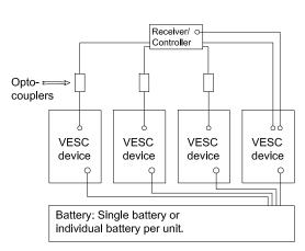
Multiple VESC controllers connected to one receiver or micro controller via PPM, UART, I²C or SPI. All devices are powered by the same battery.
