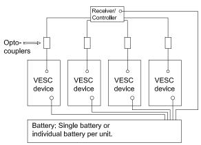
Ground loop via grid! Run computer form battery or use USB isolator.
