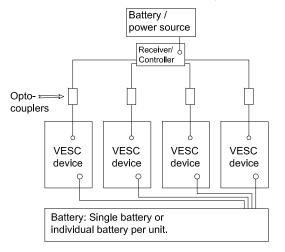
Multiple VESC controllers connected to one receiver or micro controller via PPM, UART, I<sup>2</sup>C or SPI. Receiver or micro controller is powered by one VESC device.
