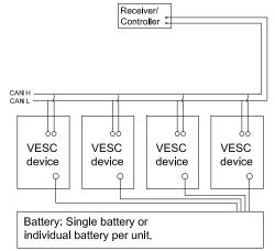
Never share any connections, other than CAN H and CAN L with other VESC devices. This will typically create a ground loop. Ground loops will damage your controllers. Only the battery ground may be shared. Use optocouplers instead.
