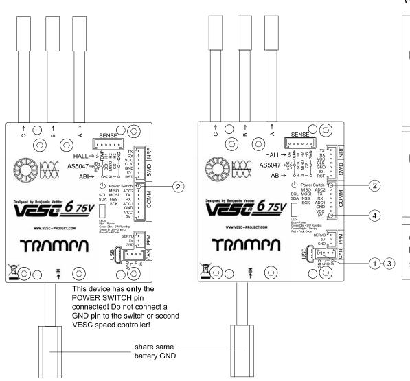
Wiring, using a Normally Closed (NC) switch
