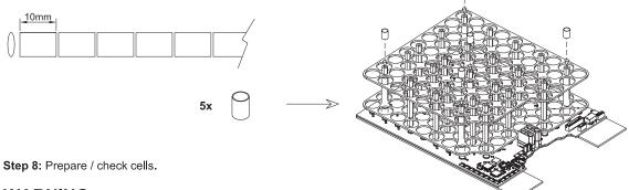
WARNING All battery cells must be of the same type, age, wear and charge level! Never use damaged cells! Shrink wrap intact?
