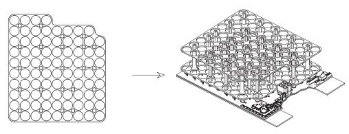
Step 7: Place 10mm long shrink tube spacers into each corner and on one central hex spacer
