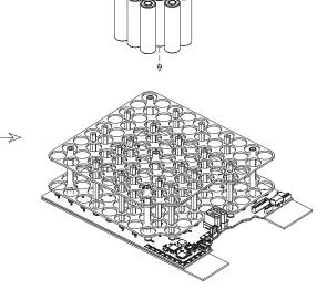
**Step 11:** After placing all cells, double check cell polarity. Use upper PCB to compare, check row by row
