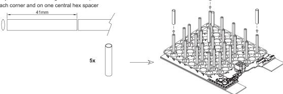
Step 6: Slide upper cell spacer into position
