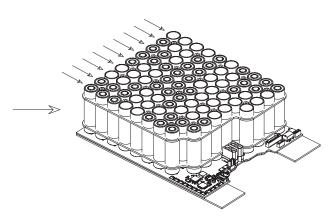
**Step 11:** <u>Clean</u> and position upper circuit board and spring panel. Use 100% alcohol to clean contacts. **CAUTION:** make sure to align the PCB carefully when presenting to the assembly! Do not shift it sideways during assembly.
