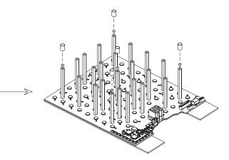
Step 4: Slide lower cell spacer into position
